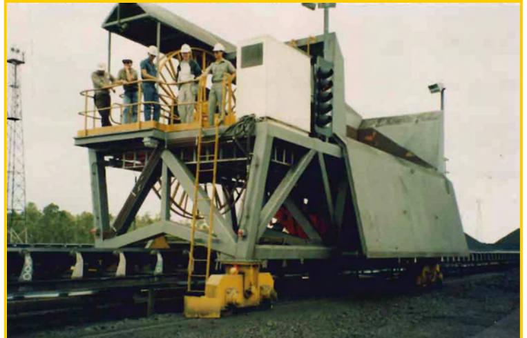
Mobile reclaim hopper car at commissioning.
